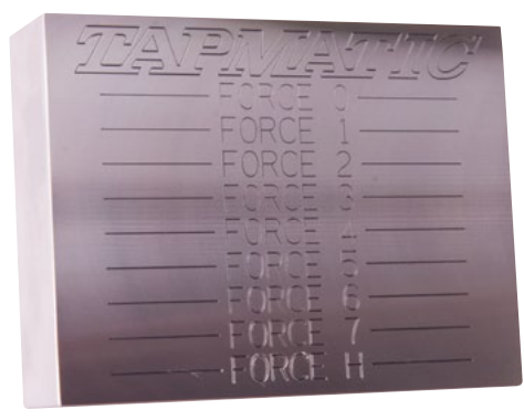
Example in 4140 pre heat treated material with hardness 28 HRC. Marking at different settings with 1.3 mm compression against the surface.
